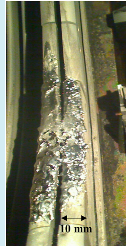
An area of melted tungsten after a disruption in the T-10 tokamak
