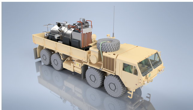
PFRC on an HEMTT for Forward Power
